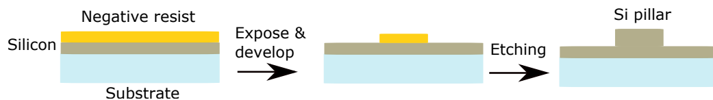
Figure 26: Schematic image of the fabrication process using a negative resist.
