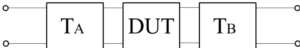
Figure 13. Measurement of a two-port DUT.
