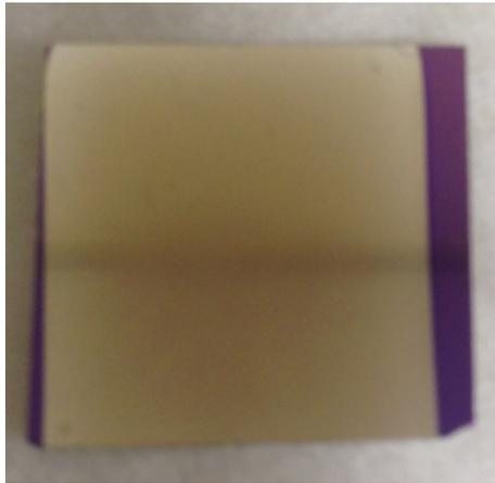
**Figura 31.** Sustrato multicapa Si-SiO-Al
