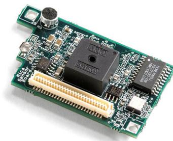
Figura 25: **Placa de sensado MTS310CA (Crossbow Technology, Inc., 2005)**
