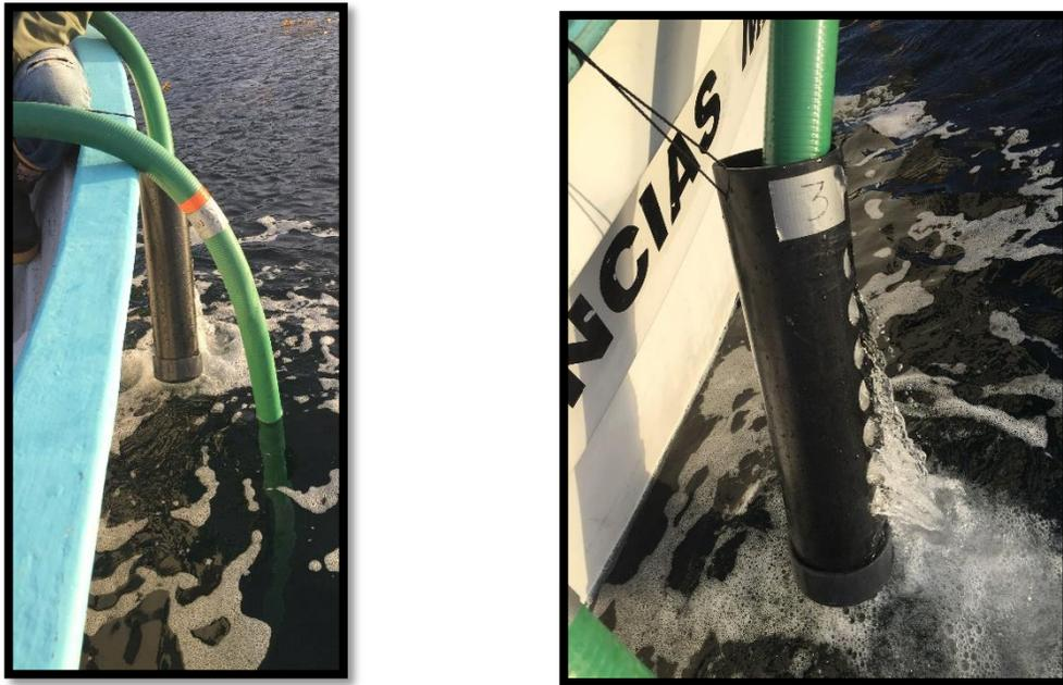
**Figure 7.** Zooplankton sampling. A hose was placed to pump water at 4 and 14 m depth (left). The other end of the hose poured water into a nytex mesh to filter zooplankton bigger than 150  $\mu\text{m}$  (right).
