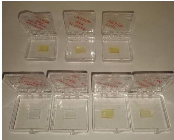
Figure 53 AR designs fabricated in CICESE using reactive thermal evaporation technique and modulation of \text{SiO}_x index to obtain three different refractive indexes similar to silica, alumina, and silicon monoxide.
