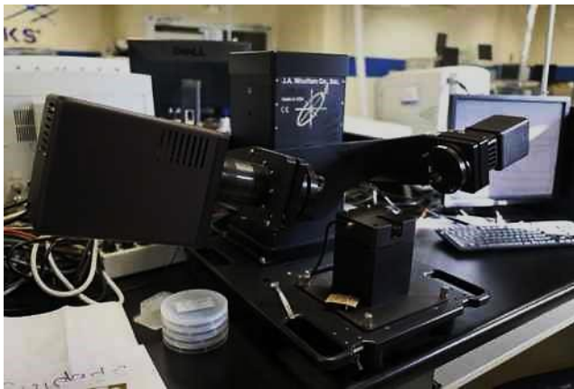
Figure 55 Ellipsometer J. A. Woollam M2000D located in the UABC campus Mexicali (left) and arrangement to perform the measurements (right).
