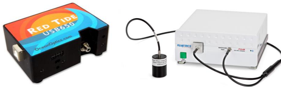
Figure 31 Spectrometers used for the characterization of the fabricated AR samples. At CICESE, was used the OceanOptics Red Tide USB650 (left) to measure the transmittance from 350 to 1000nm. On the other hand, a Filmetrics F10-AR (right) measured the spectral reflectance of the four-layer design fabricated in Corning Reynosa from 380 to 1700nm.
