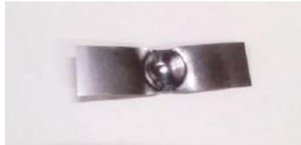
Figure 26 Molybdenum boat used to evaporate the SiO grains
