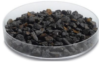
Figure 25 Grains of silicon monoxide (SiO) with a refractive index of 1.95 used for thermal evaporation; its refractive index was modulated by manipulating the synthesis parameters during evaporation.
