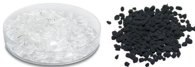
Figure 29 Pellets of \text{SiO}_2 (left) and \text{Nb}_2\text{O}_5 (right) used to make the four-layer design in the Corning Reynosa facilities.
