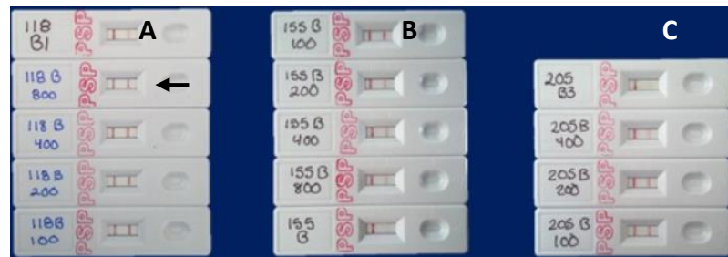
Figure 19. Scotia Rapid Testing strips obtained after dilutions. A. Profile 1. B. profile 2. C. Profile 3. The arrow points a false negative observed by analyst 2 in the dilution to 800 \mu\text{g STXeq kg}^{-1} .
