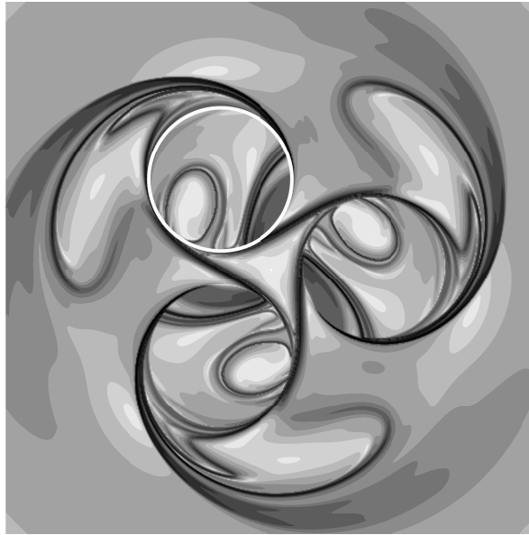
Figura 14. FTLE field in the initial condition (integration time: t = 0-2.1 ) for a Rankine-vortex trigon of relative size \alpha = 2.5 . Darker colors denote higher values of FTLE, the white circle indicates the boundary of one of the vortices.
