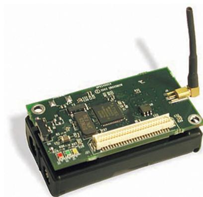
Figura 24: **Mote MICAz (Crossbow Technology, Inc., 2006b)**
