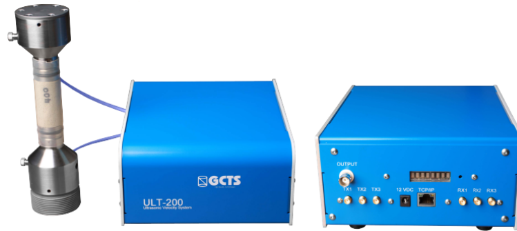
Figure 6. Ultrasonic velocity test system (ULT-200).
