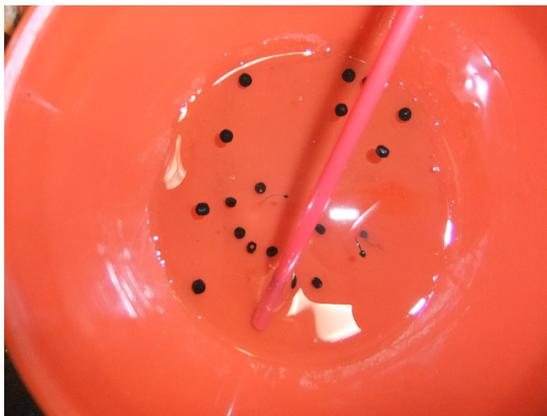
Figure 8: Colored pasta beads of anchellini used to track down flow paths
